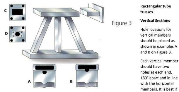
the holes are of equal size, and the combined area of the two holes at either end of the verticals should be at least 30% of the cross-sectional area.
